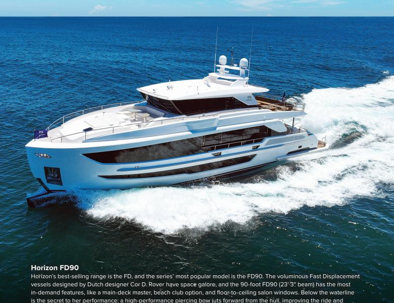
efficiency. At half-load, cruising at 10.5 knots, the FD90 has a 1,300-nautical mile range. The newest FD90, Hull No. 29, is the first one to have an open galley and a split-use skylounge, which boasts a huge covered deck behind the enclosed
